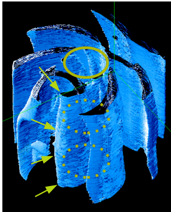
FIG. 2. Isoconcentration surfaces of the wave fronts of a vertical scroll wave in the cylinder jacket. The position of the inner tube is indicated by bright (yellow) circles. The filament of the scroll wave is located in the foreground and indicated by yellow arrows. At the side of the reactor opposite to the filament, the wave fronts are almost planar. They merge with each other, yielding almost planar fronts that propagate toward the external wall of the reactor, where they are annihilated. Sample dimensions: diameter, 21 mm; height, 15 mm.
