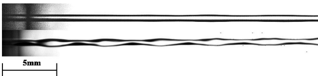
FIG. 2. Experimental observation showing the structure difference of the liquid jet from a circular (above) and elliptical (below) orifice. For comparison, the experimental conditions are well controlled. For both cases, the jet pressure is 7 kPa and the equivalent cross-section area remains the same as well.
