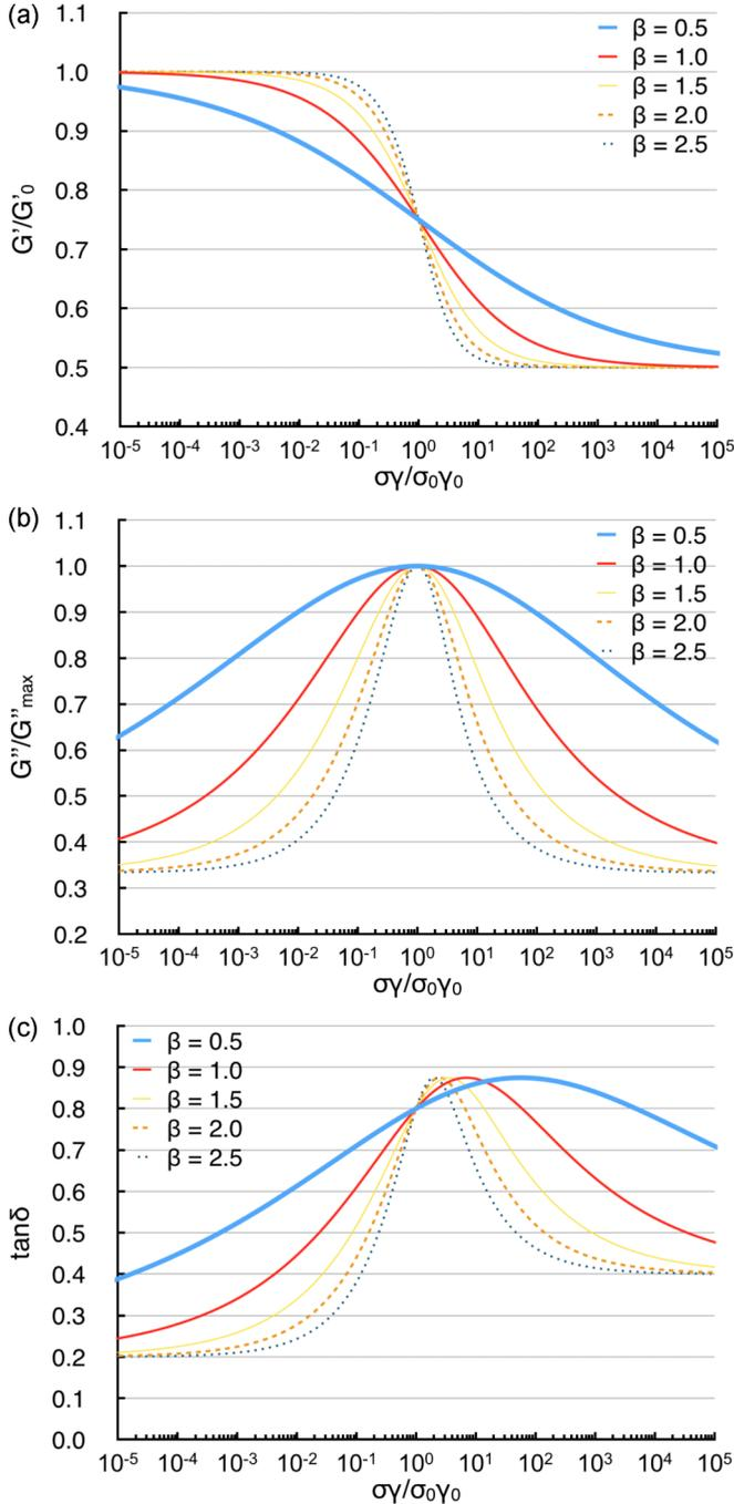
FIG. 1. Dependences of the normalized moduli (a,b) and damping factor (c) on the normalized mechanical energy density for the Kraus model.
