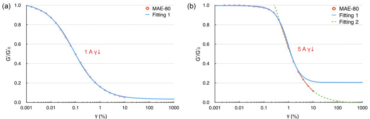
FIG. 5. Fitting of storage modulus curves at decreasing strain amplitude cycles with Kraus model for the sample MAE-80 for different driving currents:  $I = 1$  A (a) and  $I = 5$  A (b).
