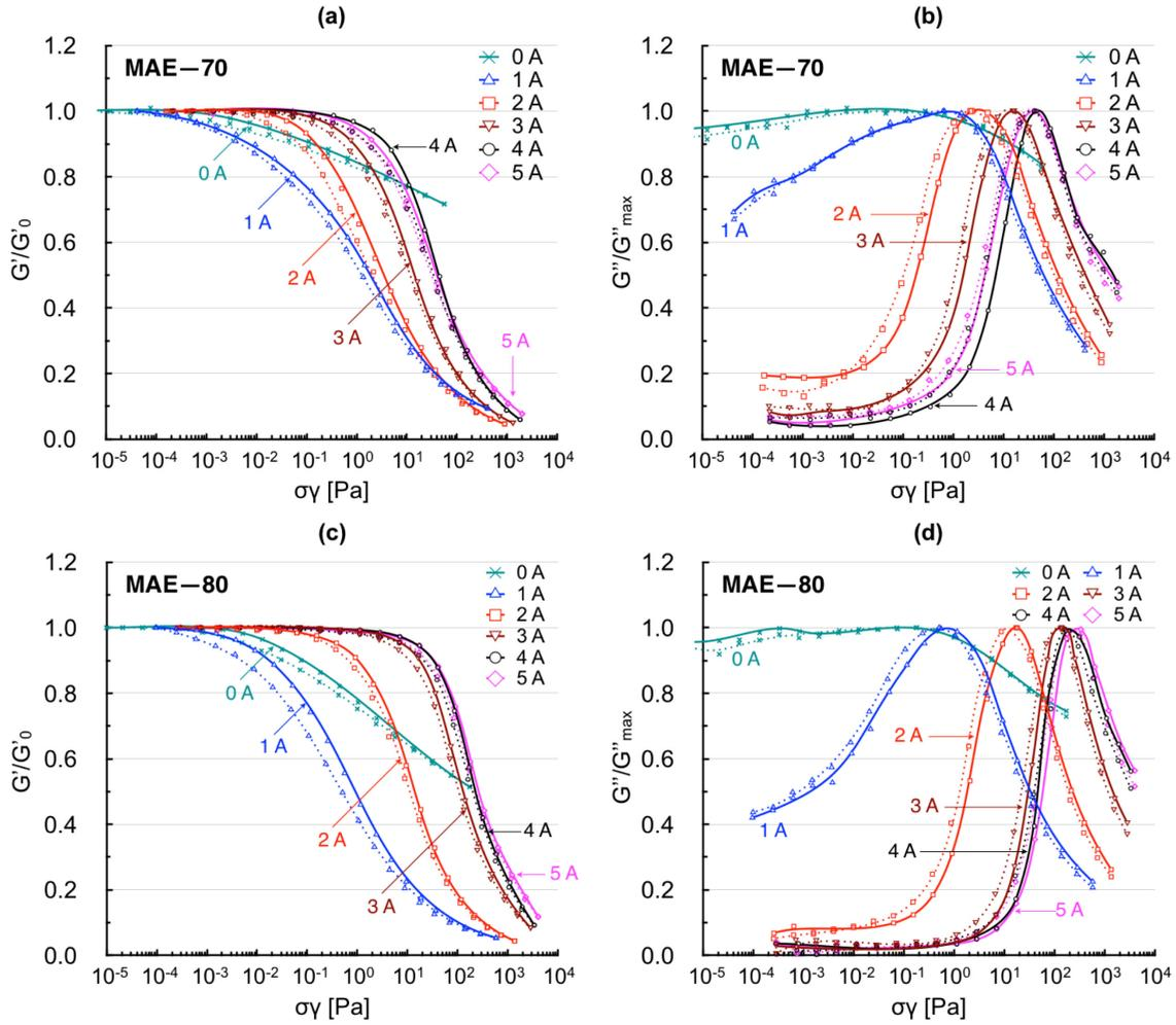
FIG. 2. Dependences of the normalized storage  $G'/G'_0$  (a,c) and loss  $G''/G''_{max}$  (b,d) moduli on the mechanical energy density  $\sigma\gamma$  for MAE-70 (a,b) and MAE-80 (c,d) samples and different drive currents  $I$  (0, 1, 2, 3, 4, and 5 A). Continuous lines denote dependencies measured with the increasing strain amplitude while dotted lines refer to the decreasing strain amplitude.
