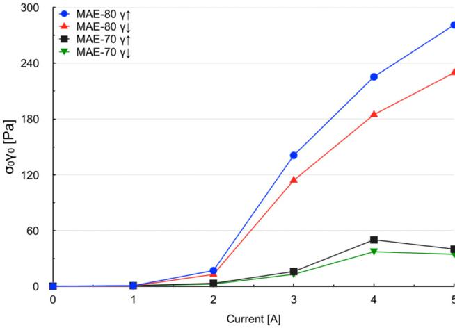
FIG. 3. Critical mechanical energy  $\sigma_0\gamma_0$  as a function of current.
