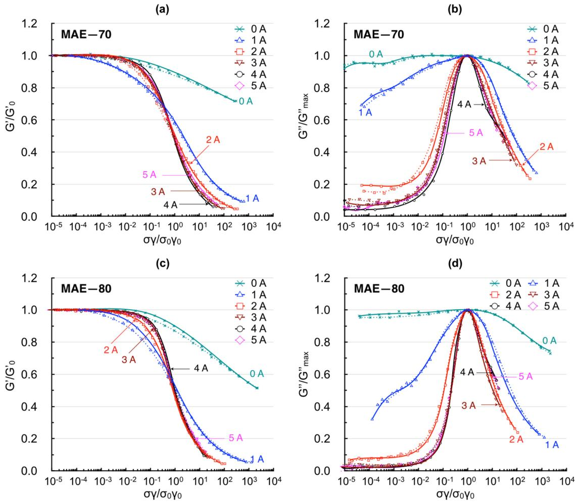
FIG. 4. Dependences of the normalized shear storage  $G'/G'_0$  (a,c) and loss  $G''/G''_{max}$  (b,d) moduli on the normalized mechanical energy  $(\sigma\gamma)/(\sigma_0\gamma_0)$  for the MAE-70 (a,b) and MAE-80 (c,d) samples at different drive currents  $I$  (0, 1, 2, 3, 4, and 5 A). Continuous lines denote dependencies measured with the increasing strain amplitude while dotted lines refer to the decreasing strain amplitude.
