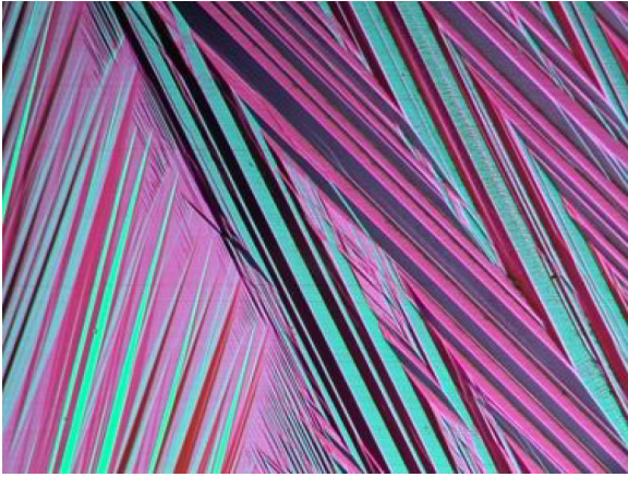
FIG. 1. Example of the final microstructure on a \text{Cu}_{69.3}\text{Zn}_{17}\text{Al}_{13.7} single crystal, after the thermally induced transformation from cubic to monoclinic phase is completed. The image corresponds to a \sim 8\text{ mm} \times 6\text{ mm} area approximately perpendicular to the the [100] direction. It has been obtained by using polarized light on a sample initially polished in the cubic phase. Different colors indicate slightly different orientations of the sample surface and, therefore, approximately correspond to different variants.
