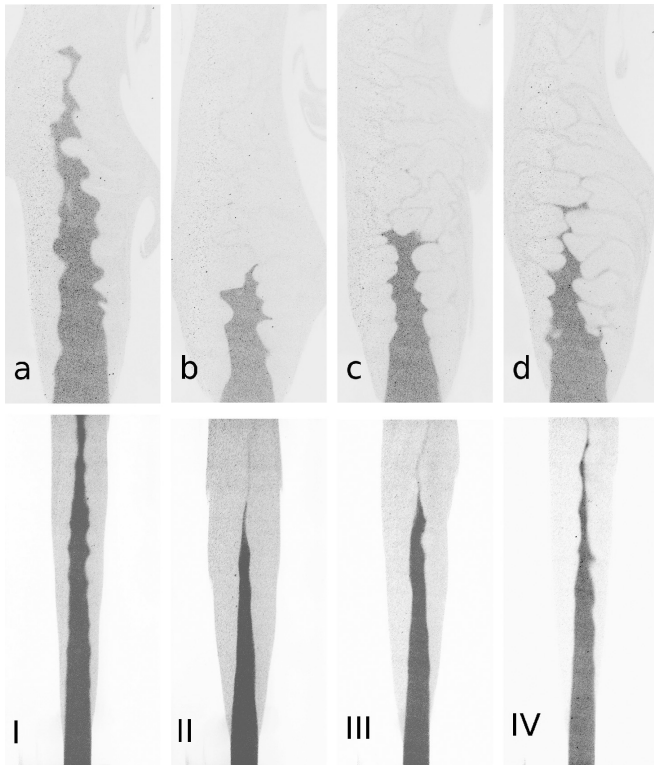
FIG. 10. Mie scattering images of \text{C}_3\text{H}_8/\text{Air} flames at \text{Re} = 5000 . Upper panels: Bunsen diameter L = 18 \text{ mm} . Lower panels: L = 9 \text{ mm} . Flames a-d and I-IV correspond to \phi = 0.8, 1.1, 1.4, 1.5 , respectively.
