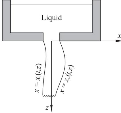
FIG. 1. The setting: a free-falling liquid curtain.
