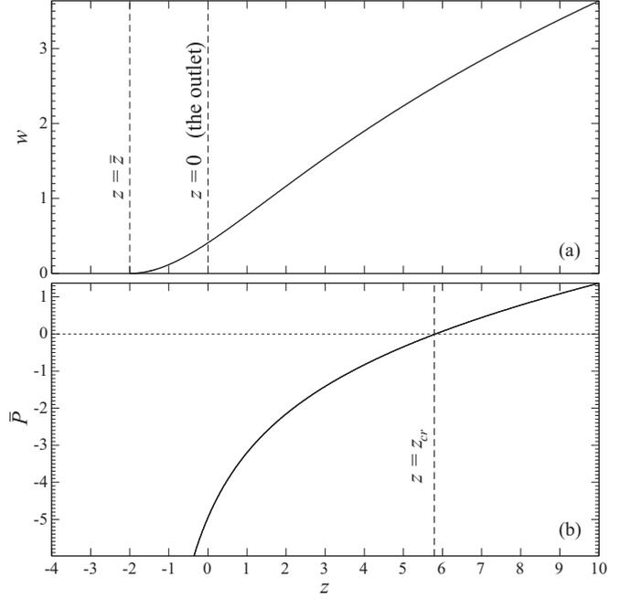
FIG. 2. The solution of the boundary-value problem (35)–(37) for  $\bar{z} = -2$ . The curtain's outlet is located at  $z = 0$ . (a)  $\bar{w}$  vs  $z$ ; (b)  $\bar{P}$  [defined by (41)] vs  $z$ .  $z_{\text{cr}}$  is the coordinate of the critical point such that  $\bar{P}(z_{\text{cr}}) = 0$ .
