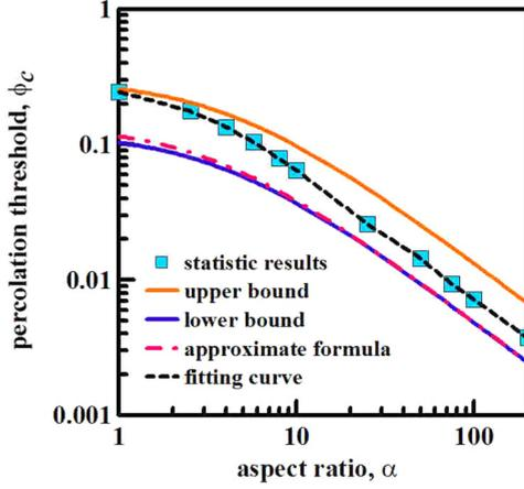
FIG. 5. The percolation threshold  $\phi_c$  for different  $\alpha$ . The cubic symbols are the present MC simulation results, the solid lines are theoretical bounds for the percolation threshold of congruent overlapping spherocylinders derived by Torquato and Jiao [16], and the dashed red line is the approximate solution for the percolation threshold reported by Chatterjee [11].
