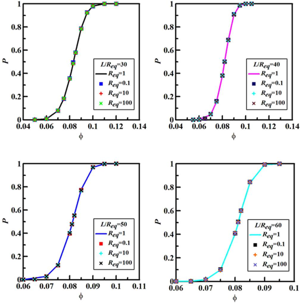
FIG. 8. Percolation probability  $P(\phi, L)$  versus  $\phi$  for different  $R_{eq}$  and system sizes of  $L$ . The parameters of the particles are  $\alpha = 8.0$ .
