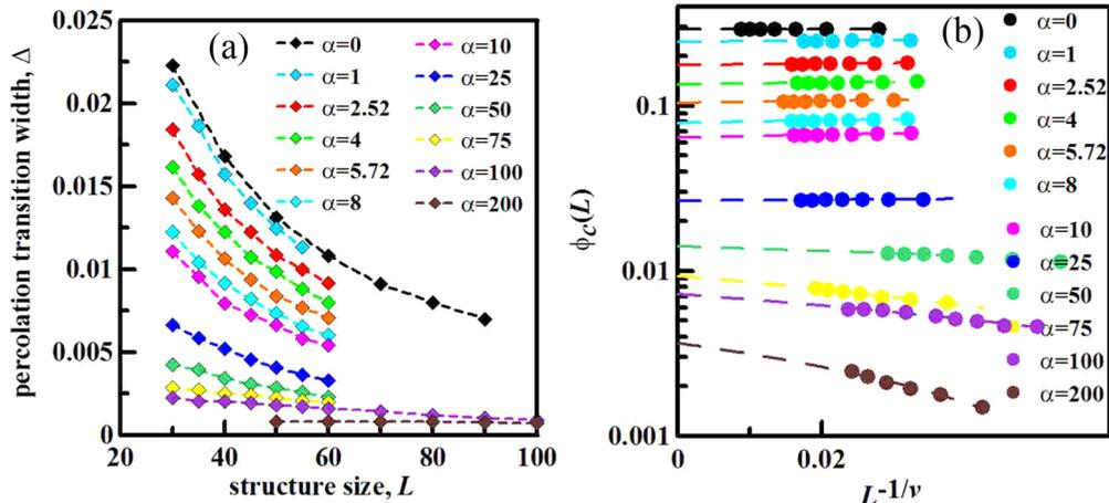
FIG. 4. (a) The percolation transition width  $\Delta$  for different  $\alpha$  as a function of system size  $L$ . (b) The effective percolation threshold  $\phi_c(L)$  for different  $\alpha$  as a function of  $L^{-1/\nu}$ , with linear fits to the data.
