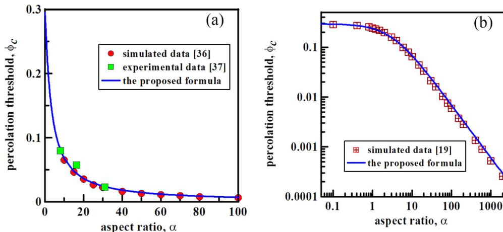
FIG. 7. Comparisons of the proposed empirical approximation with (a) the numerical and experimental results from Mutiso and coworkers [36,37], and with (b) the numerical results from Schilling *et al.* [19].
