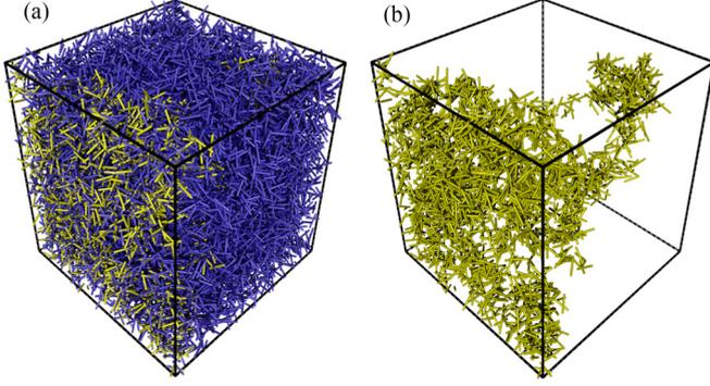
FIG. 1. (a) Realization of a congruent overlapping spherocylinder system with the aspect ratio of  $\alpha = 8$ ; (b) identification of a percolating cluster in the system.
