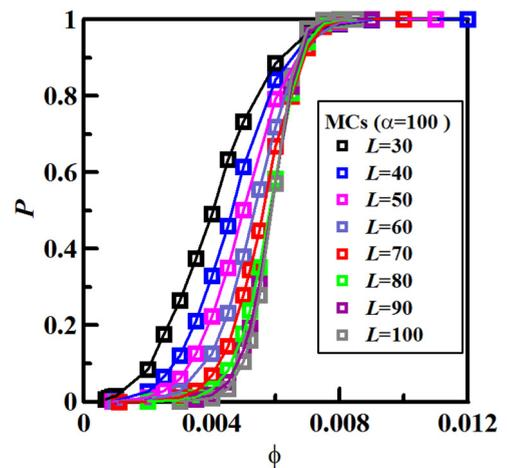
FIG. 2. Percolation probability  $P$  for different sizes  $L$  of cubic domain as a function of  $\phi$  for congruent overlapping spherocylinders. The parameters of the particles are  $R_{\text{eq}} = 1.0$  and  $\alpha = 100.0$ . The cubic symbols are MC simulation results and the lines are fitting results. The percolation probability curves for various  $\alpha$  are displayed in Fig. 3.
