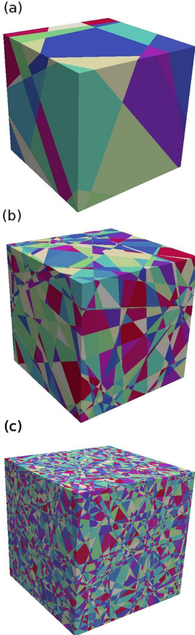
FIG. 2. Examples of Monte Carlo realizations of isotropic Poisson geometries restricted to a three-dimensional box of linear size L . For all realizations, we have chosen L = 20 . The geometry at (a) the top has \lambda = 0.2 , that at (b) the middle has \lambda = 1 and that at (c) the bottom has \lambda = 3 . For fixed L , the average number of random polyhedra composing the geometry increases with increasing \lambda .
