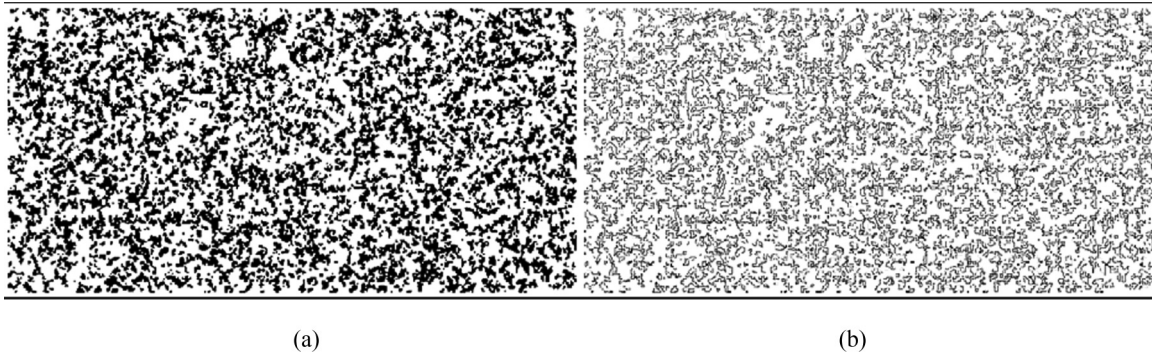
FIG. 2. Disordered random porous media reconstructed with the QSGS and BRCP (a) the phase image and (b) the boundary recognition. The domains are 1008 \times 520 lattice units in size.
