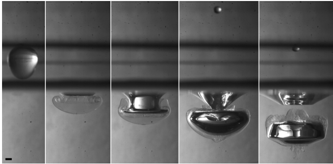
FIG. 11. Large bubble entrapment for a drop of 6% \text{MgSO}_4 , giving \rho_d/\rho_p = 1.06 and \mu_d = 1.3 cP for D = 5.0 mm, V = 0.94 m/s, and H = 5.0 cm. The sequence shows the following times: -2.3, 7, 11, 17, and 25 ms after the first contact. The scale bar is 1 mm long.
