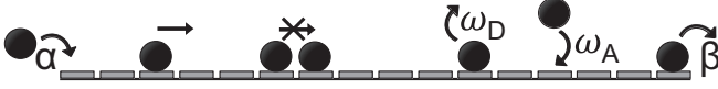
FIG. 1. Schematic of the TASEP model with LK. Particles are injected at the first site with rate \alpha and extracted at the last site with rate \beta . The motion of particles is totally asymmetric as they move exclusively to the right with a unitary rate given that the site is empty. Hopping over an occupied site is not allowed. Pure TASEP is composed of injection, extraction, and asymmetric hopping of particles interacting via hard-core repulsion. In the TASEP + LK model, LK are additionally included by allowing particles to detach from an occupied site with rate \omega_D and attach to an unoccupied site with rate \omega_A .
