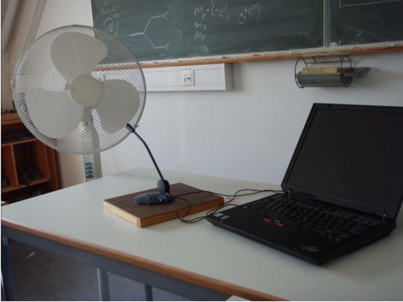
FIG. 2. (Color online) Setup for the generation and measurement of the turbulent air flow. The turbulent air flow has been generated by the fan on the left hand side and recorded by the microphone in front of it. In the preliminary stage of the experiments, the sound card of the laptop has been used for data acquisition.
