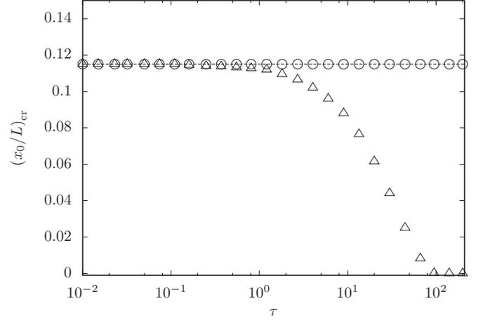
FIG. 4. Critical value of  $x_0/L$  as a function of the delay  $\tau$  introduced after the reset. Results are shown both for the case of *resetting subordinated to motion* (triangles) and *resetting independent of motion* (circles) to observe the different dynamics that the delay induces in each case. Arbitrary values  $v_0 = 1$  and  $L = 200$  have been used in all the cases.
