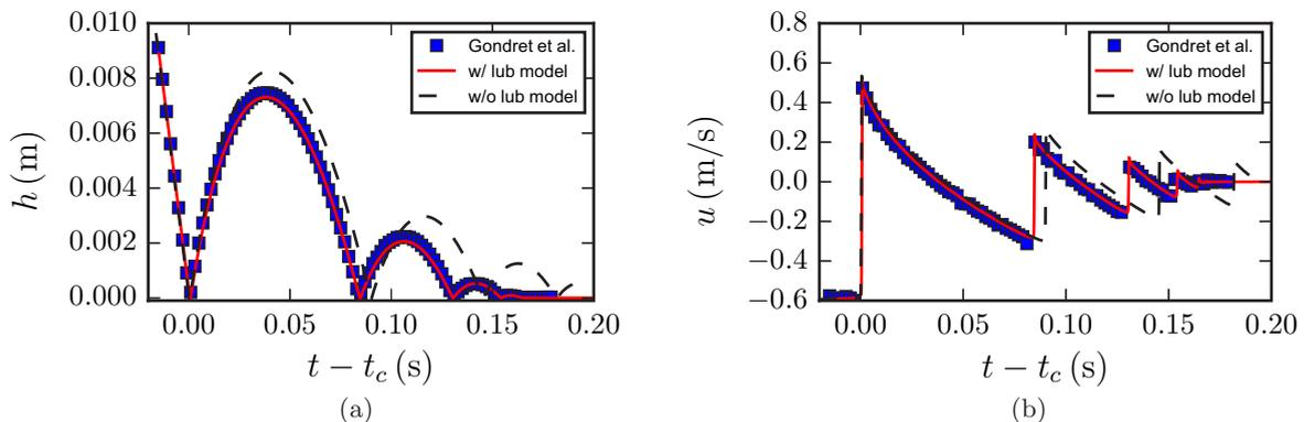
FIG. 6. (Color online) Trajectory (a) and time evolution of the particle velocity (b) in the bouncing motion of a steel sphere colliding onto a planar surface in silicon oil RV10.
