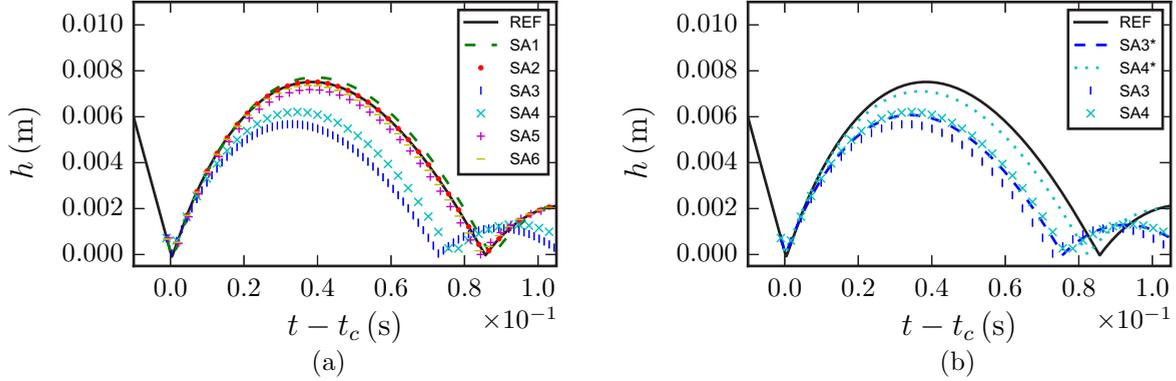
FIG. 8. (Color online) Sensitivity analysis to the time step, substepping, and stretching of the collision time (a) and outcome of cases SA3 and SA4 when problematic Lagrangian forcing points are excluded from the IBM forcing scheme (b). Computational parameters in Table III.
