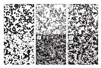
FIG. 2. Boolean models of overlapping grains for (a) circles, (b) ellipses, and (c) rectangles. A set of N points is selected randomly in a plane (total area  $L^2$ ) (Poisson process). At each point a grain with random orientation is placed. Each structure is characterized by its point density  $N/L^2$ . The white phase corresponds to the conducting phase. (a)–(c) are structures, which we classify as void percolation, whereas the structures (d)–(f) exhibit grain percolation.
