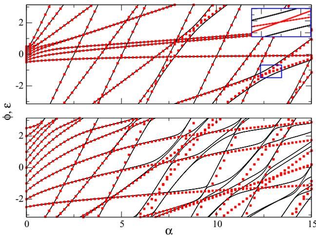
FIG. 1. (Color online) Quasienergy spectrum (solid line) of the Floquet operator  $\widehat{\mathcal{F}}$  and the energy eigenvalues (solid square) of the effective Hamiltonian  $\widehat{H}_{\text{eff}}$  are compared as a function of  $\alpha$ . Upper window shows the result for  $\beta = 0.1$ , and the lower window shows the same for  $\beta = 0.5$ . Whereas the integrable  $\widehat{H}_{\text{eff}}$  shows level crossing, the quasienergy spectrum indicates level repulsion (see inset).
