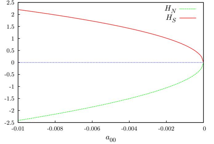
FIG. 5. (Color online)  $H_N$  (dashed green) and  $H_S$  (solid red) vs  $a_{00}$  for the perturbation  $h$  characterized by two modes  $a_{00}$  and  $a_{10}$ . The above plot is for the case when  $a_{10} < 0$ , which corresponds to the inward buckling of the north pole. See text for the meaning of the symbols.
