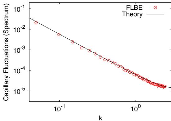
FIG. 6. (Color online) Capillary fluctuations of a planar one-dimensional interface obtained with mean-field lattice interactions (see Sec. VIB). The equal-time spectrum of interfacial height fluctuations obtained from LBE simulations (circles) is compared with the theoretical structure factor (solid line) reported in Eq. (91). The wave vector in the interface region is indicated with  $k$ . Simulation parameters are reported in the text.
