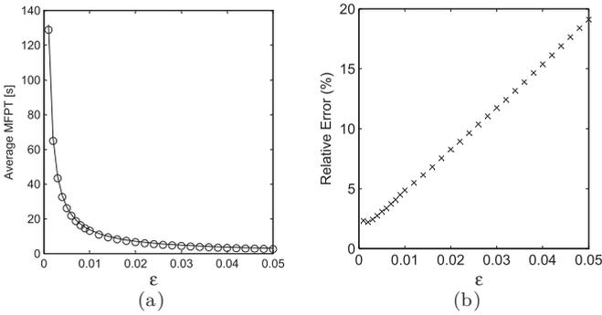
FIG. 7. Plots of (a) comparison of numerical (circles) and two-term asymptotic expression for average MFPT, and (b) relative error [see (22)] for a prolate spheroid with  $N = 5$ .
