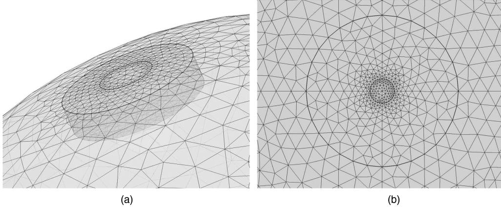
FIG. 2. Illustration of extremely fine and fine mesh regions.
