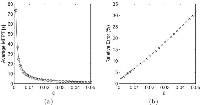
FIG. 3. Plots of (a) comparison of numerical (circles) and two-term asymptotic expression for average MFPT, and (b) relative error [see (22)] for an oblate spheroid with  $N = 3$ .
