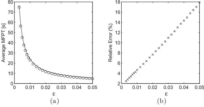
FIG. 6. Plots of (a) comparison of numerical (circles) and two-term asymptotic expression for average MFPT, and (b) relative error [see (22)] for a prolate spheroid with  $N = 3$ .
