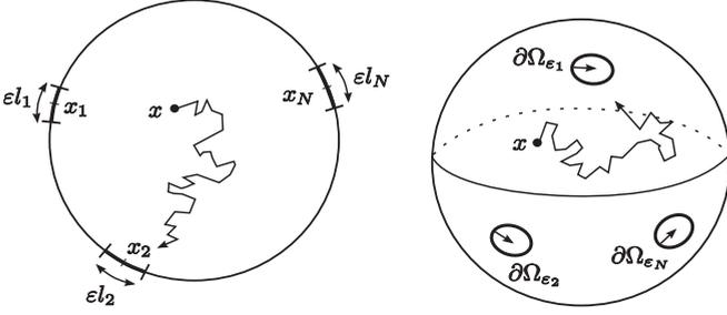
FIG. 1. A schematic of the narrow escape problem in a two- and a three-dimensional domain.
