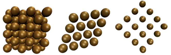
FIG. 1. (Color online) Left: FCC crystal with C = 3 cubic unit cells along each edge. Center: Rhombic (111) FCC patch with P = 4 atoms along each edge. Right: Square (100) FCC patch with P = 4 atoms along each edge.
