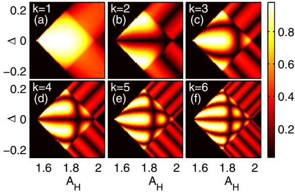
FIG. 3. (Color online) Numerical simulation: The normalized response amplitude  $R_{L, \text{norm}}^{(k)}$  of a bistable system on the frequency  $f_k = kf_L$  versus the level of asymmetry  $\Delta$  and the HF amplitude  $A_H$  ( $f_L = 0.001$ ,  $f_H = 0.1$ ).
