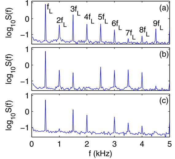
FIG. 1. (Color online) Experiment: Amplitude spectrum  $S(f)$  of the laser response on the selected polarization shown for three different values of  $A_H$ :  $j_{dc} = 17.44$  mA;  $A_H = 78$  (a), 87 (b), 98 (c) mV.
