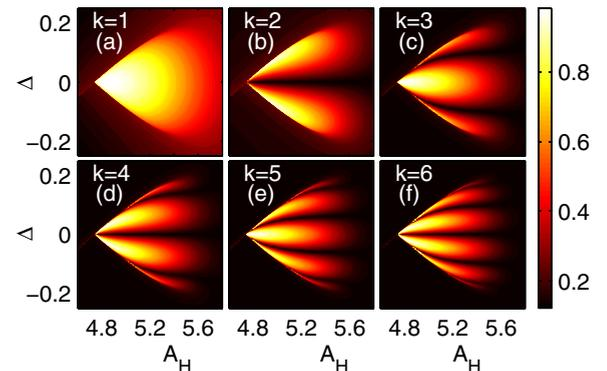
FIG. 9. (Color online) Numerical simulation: The normalized response amplitude  $R_{L, \text{norm}}^{(k)}$  of a bistable system on the frequency  $f_k = kf_L$  versus the level of asymmetry  $\Delta$  and the HF amplitude  $A_H$  ( $f_L = 0.01$ ,  $f_H = 1$ ).
