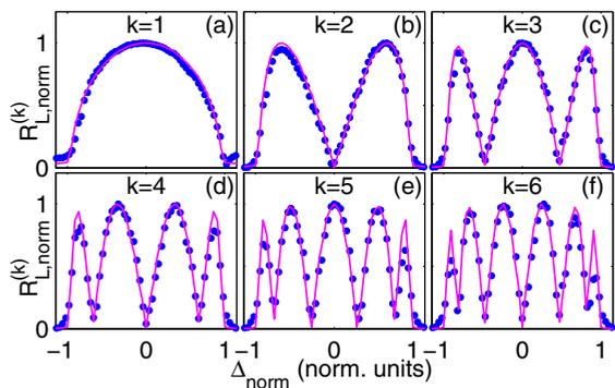
FIG. 4. (Color online) The normalized response amplitude  $R_{L, \text{norm}}^{(k)}$  versus normalized level of asymmetry  $\Delta_{\text{norm}}$ . The amplitude of the HF signal  $A_H = 68.6$  mV (experiment) and 1.77 (numerical simulation). Points, the experiment; solid line, the numerical simulation.
