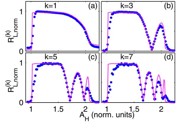
FIG. 5. (Color online) The normalized response amplitude  $R_{L, \text{norm}}^{(k)}$  versus normalized amplitude of HF signal  $A_H$  for the symmetrical configuration of a bistable potential. Points, the experiment; solid line, the numerical simulation.
