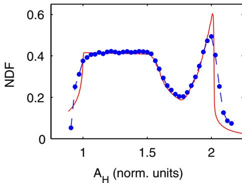
FIG. 7. (Color online) The nonlinear distortion factor  $\chi$  versus the normalized HF amplitude  $A_H$  for the case of a symmetrical configuration of a double-well potential. Points, experiment; solid line, simulation.
