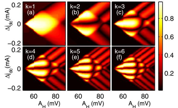
FIG. 2. (Color online) Experiment: The normalized laser response amplitude  $R_{L,\text{norm}}^{(k)}$  on the frequency  $f_k = kf_L$  ( $k = 1, 2, \dots, 6$ ) versus the level of asymmetry  $\Delta j_{dc}$  and the HF amplitude  $A_H$ .
