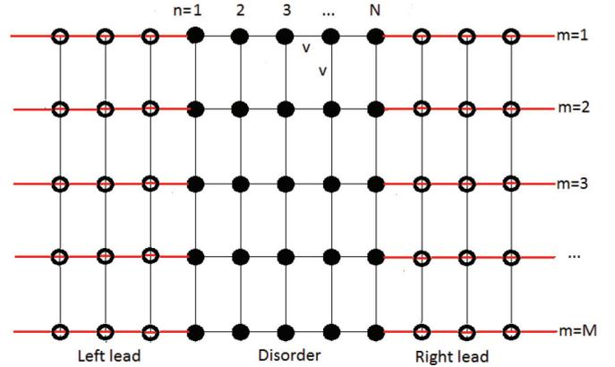
FIG. 1. (Color online) Disordered Q1D wire of length  $N$  and width  $M$  (full circles) connected at both ends to semi-infinite ideal leads of width  $M$  (open circles).
