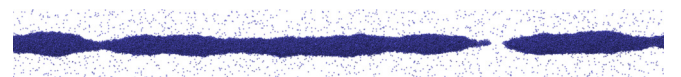
FIG. 3. (Color online) A typical profile obtained during simulation (set 2, 260 ps into the production run). The irregular beadlike fluid structure, which eventually breaks up into pieces of varying sizes, can be seen clearly.
