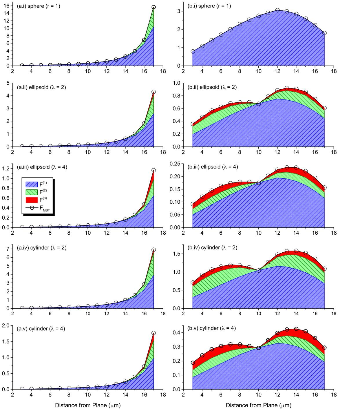
FIG. 6. (Color online) Stacked area plots showing the first three terms of DEP force ( $F^{(1)}$ ,  $F^{(2)}$ , and  $F^{(3)}$ ) and the total DEP force ( $F_{MST}$ ), determined numerically, on (i) spherical ( $r = 1 \mu\text{m}$ ), ellipsoidal [(ii)  $\lambda = 2$ , (iii)  $\lambda = 4$ ], and cylindrical [(iv)  $\lambda = 2$ , (v)  $\lambda = 4$ ] particles in (a) point-plane and (b) disk-plane electrode configurations.
