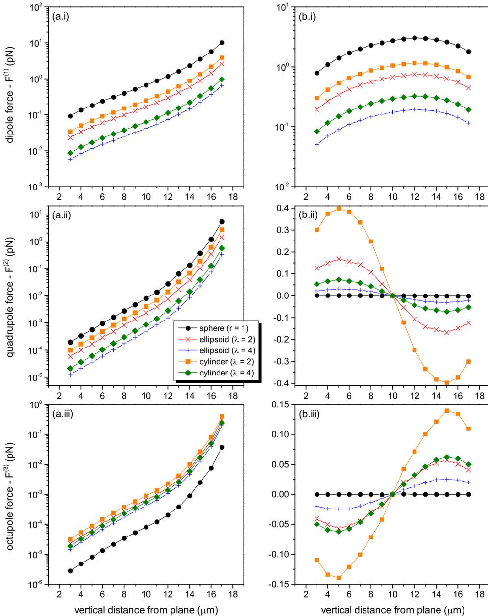
FIG. 4. (Color online) (i) First- ( $F^{(1)}$ ), (ii) second- ( $F^{(2)}$ ), and (iii) third-order ( $F^{(3)}$ ) terms of DEP force on spherical ( $r = 1 \mu\text{m}$ ), ellipsoidal ( $\lambda = 2, \lambda = 4$ ), and cylindrical ( $\lambda = 2, \lambda = 4$ ) particles at different positions along the symmetry axes of (a) point-plane and (b) disk-plane electrode structures.
