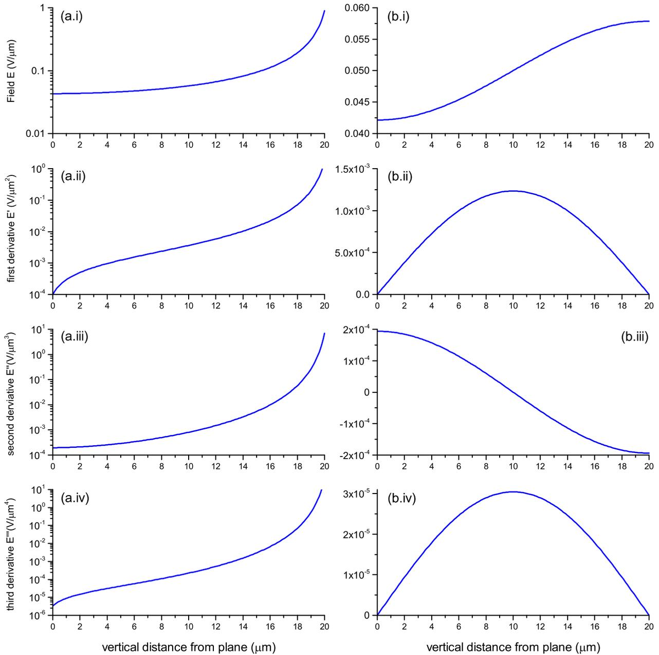
FIG. 2. (Color online) Field curvature profiles for point-plane and disk-plane electrode structures showing the pronounced effect of electrode design on electric field nonuniformity: (i) the electric field magnitude and its (ii) first-, (iii) second-, and (iv) third-order derivatives along the symmetry axes of (a) point-plane and (b) disk-plane electrode structures with the characteristics given in Fig. 1.
