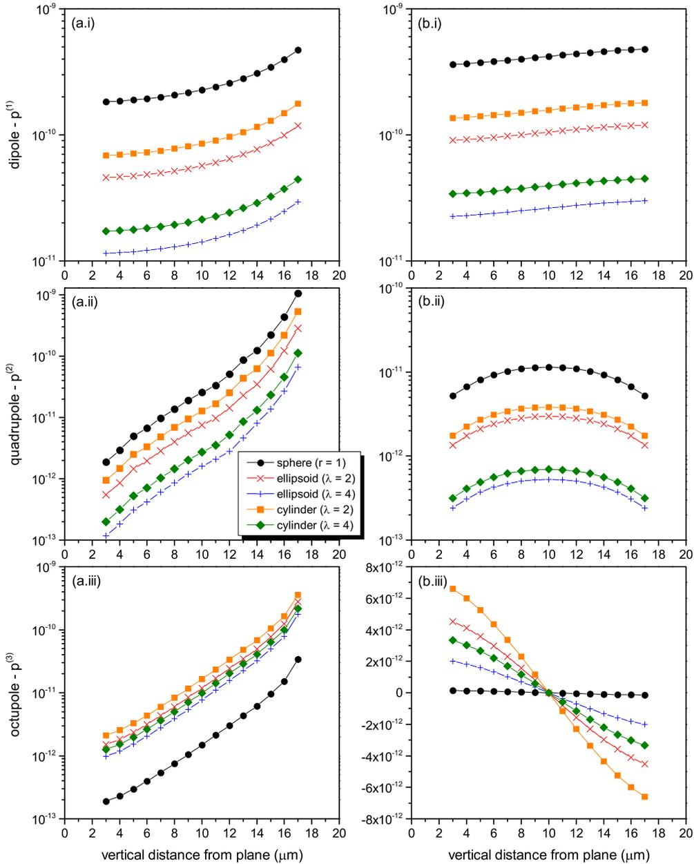
FIG. 3. (Color online) (i) First- ( $p^{(1)}$ ), (ii) second- ( $p^{(2)}$ ), and (iii) third-order ( $p^{(3)}$ ) effective moments of spherical ( $r = 1 \mu\text{m}$ ), ellipsoidal ( $\lambda = 2, \lambda = 4$ ), and cylindrical ( $\lambda = 2, \lambda = 4$ ) particles at different positions within (a) point-plane and (b) disk-plane electrode structures.
