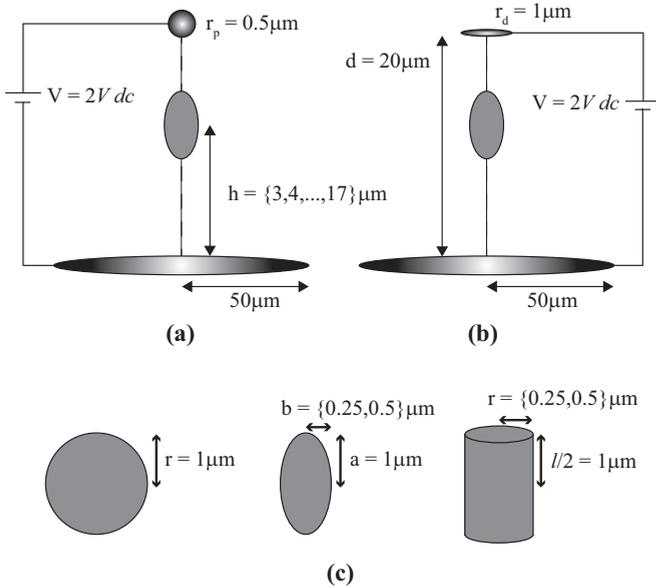
FIG. 1. Electrode structures and particle shapes and dimensions studied in this work for analysis of the effect of electrode or field and particle geometry on the significance of higher-order DEP forces: (a) the point-plane electrode structure, (b) the disk-plane electrode structure, (c) dimensions of spherical, ellipsoidal, and cylindrical particles.
