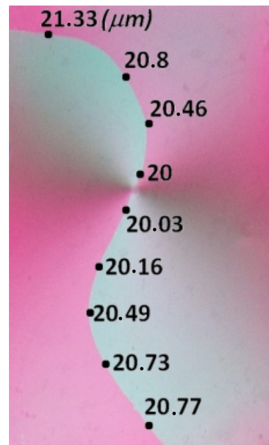
FIG. 4. (Color online) Photograph of the cell with inhomogeneous thickness in crossed polarizers. The cells filled with composition 5CB and S-811: c = 3.7 \times 10^{-3} . The numbers indicate the local thickness of the cell. The dimension of the picture is 1 \times 2 \text{ cm} . The calculated thickness of the cell along the disclination line is depicted on the figure.
