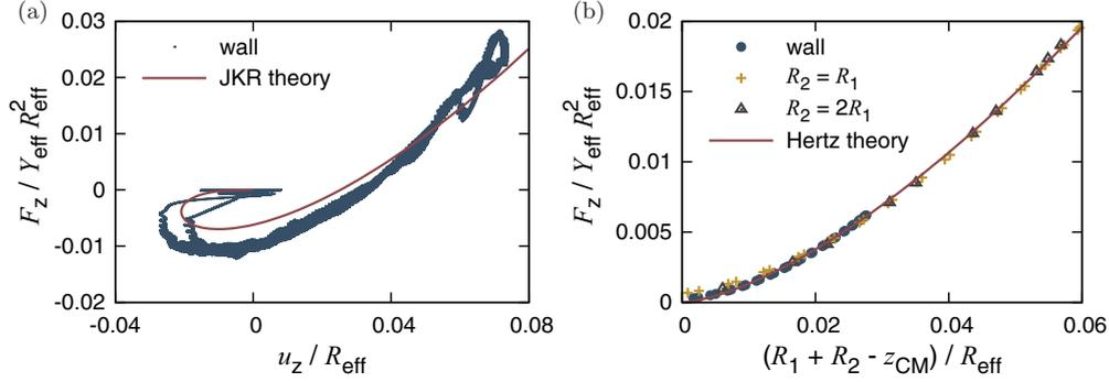
FIG. 7. (Color online) The scaled force as a function of the displacement at the pole  $(r, \theta, \phi) = (R_1, 0, 0)$  without the solid viscosity for (a) the attractive ( $g = 1$ ) and (b) the repulsive ( $g = 0$ ) cases, respectively. Here, “wall” represents the results of simulation for collision between the sphere and the wall.
