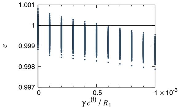
FIG. 10. (Color online) The restitution coefficient against the solid viscosity  $\gamma$  for the impact speed  $v_{\text{CM}}(0) = 0.009c^{(t)}$ .
