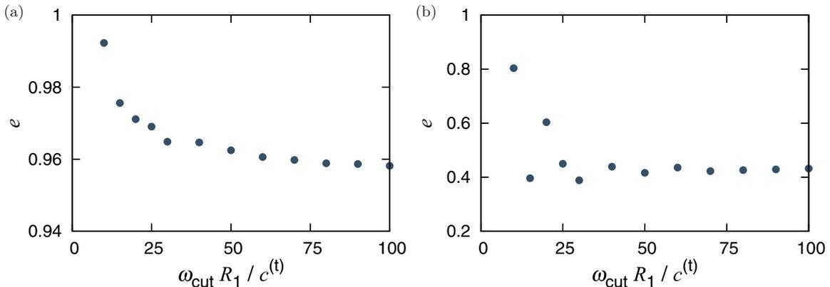
FIG. 2. (Color online) The cutoff frequency  $\omega_{\text{cut}}$  dependence of the restitution coefficient for  $T = 0$ ,  $\gamma = 0$ , and (a)  $v_{\text{CM}}(0) = 0.1c^{(l)}$  and (b)  $v_{\text{CM}}(0) = 0.01c^{(l)}$ .
