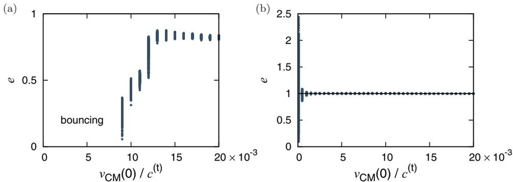
FIG. 8. (Color online) The impact speed dependence of the restitution coefficient for  $T = 2.14 \times 10^{-8} M(c^{(t)})^2$  case with fixing (a)  $g = 1$  and (b)  $g = 0.2$ , respectively. The temperature corresponds to 300 K in the physical unit.
