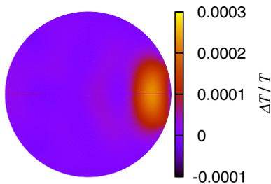
FIG. 13. (Color online) The heating distribution on the cross section at the instant of the impact for  $v_{\text{CM}} = 0.1$ . It should be noted that the heat distribution is plotted at the position of an undeformed sphere.
