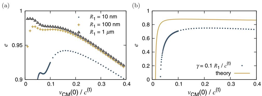
FIG. 6. (Color online) The restitution coefficient against the impact speed for (a)  $\gamma = 0.01 R_1/c^{(t)}$  and (b)  $\gamma = 0.1 R_1/c^{(t)}$ , respectively. The solid line in (b) represents the theoretical prediction of cohesive collisions between viscoelastic spheres.
