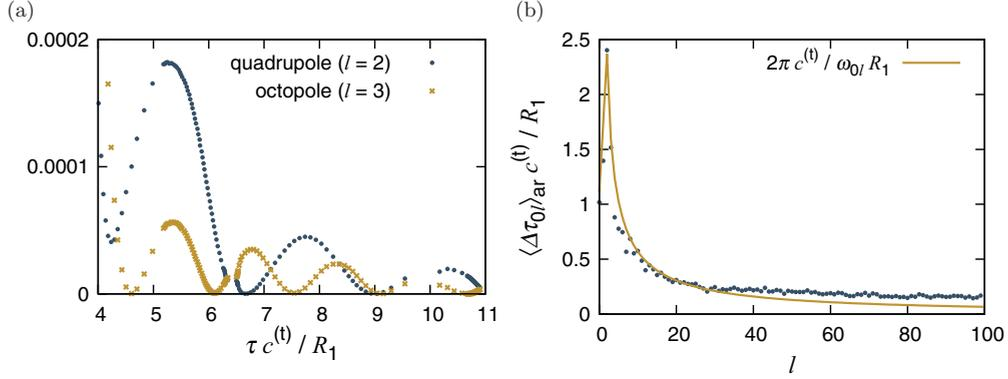
FIG. 5. (Color online) (a) The excitation of the quadrupole and the octopole modes against the contact duration and (b) the arithmetic mean of the intervals  $\langle \Delta \tau_{0\ell} \rangle_{ar}$  between the local minima of  $\Delta H_{0l0}(\tau)$  for all the fundamental modes. The solid line in (b) represents the inverse of eigenfrequencies  $2\pi/\omega_{0\ell}$ .
