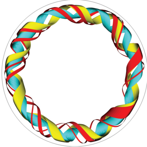
FIG. 9. (Color online) Examples for KAM tubes with larger winding numbers for Re = 1800 : T_{1a,b}^8 [red (dark)], T_3^9 [yellow (bright)], and T_{1a}^{10} [cyan (medium gray)]. The circle indicates the free surface.
