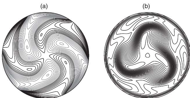
FIG. 4. Equidistant isolines of the azimuthal velocity (a) in the laboratory frame of reference and of the temperature field (b) at midplane z = 0 for the fully developed clockwise-traveling hydrothermal wave for Re = 1800 . Gray isolines indicate negative values.
