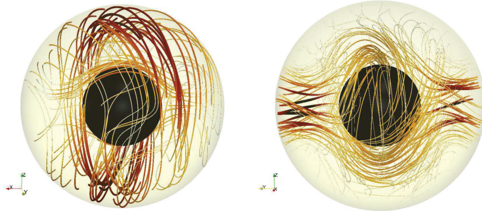
FIG. 3. (Color online) Magnetic eigenmodes close to the onset for kinematic dynamo action driven by the S_2^2 T_2^2 reversible flow. Left: The boundary conditions are perfectly conducting (no normal field). Right: The boundary conditions correspond to a pseudovacuum (no tangent field). In both cases, the magnetic field is dominated by a strong m = 1 mode. The magnetic field lines are initiated randomly in the spherical shell. The dark and thick magnetic field lines correspond to large magnetic field amplitude, whereas bright and thin lines correspond to low magnetic field magnitude. The growth rate associated with these two eigenmodes is exactly the same.
