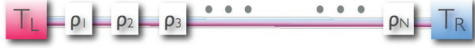
FIG. 2. (Color online) The model is defined on lattice sites, each one characterized by an energy \rho_l . The dynamics is stochastic and proceeds via random collisions between nearest neighbors where part of the pair energy is dissipated to the environment and the rest is randomly redistributed within the pair. Such dynamics mimics at the mesoscopic level the evolution of a wide class of systems characterized by a nontrivial competition between diffusion and dissipation.
