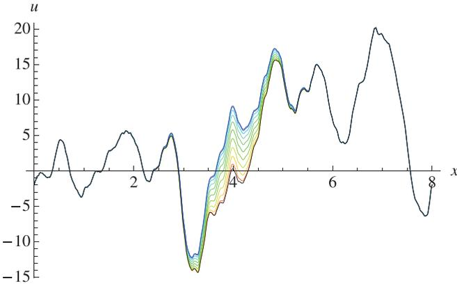
FIG. 6. (Color online) Disorder-averaged unfolding of an avalanche following a local step in the force at  $x_0 = 4$  and of duration  $T = 1$ , according to formula (281). Mean intermediate positions  $u(x, t = 0) + \int_0^t \langle \dot{u}_{xt} \rangle_{0T}$  are shown at  $t$  multiples of  $T/10$ . The velocity  $\dot{u}_{xt} \geq 0$ , so the motion is towards the top of the plot. For the sake of illustration we chose a random but fixed initial condition  $u(x, t = 0)$ .
