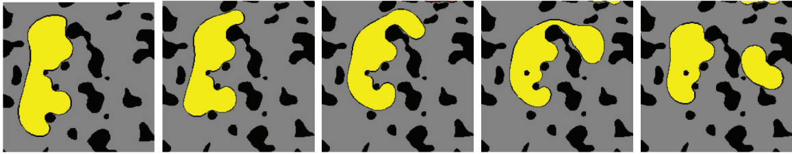
FIG. 7. (Color online) A sequence of snapshots focusing on a subdomain where N+ events commonly occur during the numerical simulation. A significant structural deformation of the original blob as it goes through a narrower pore leads to a N+ event. S_{nw} = 0.2 , Bo = 0.127 , \lambda_s = 15\delta x . Nonwetting phase blobs are shown in yellow (brighter color in gray scale), wetting phase in gray, and solid sites in black.
