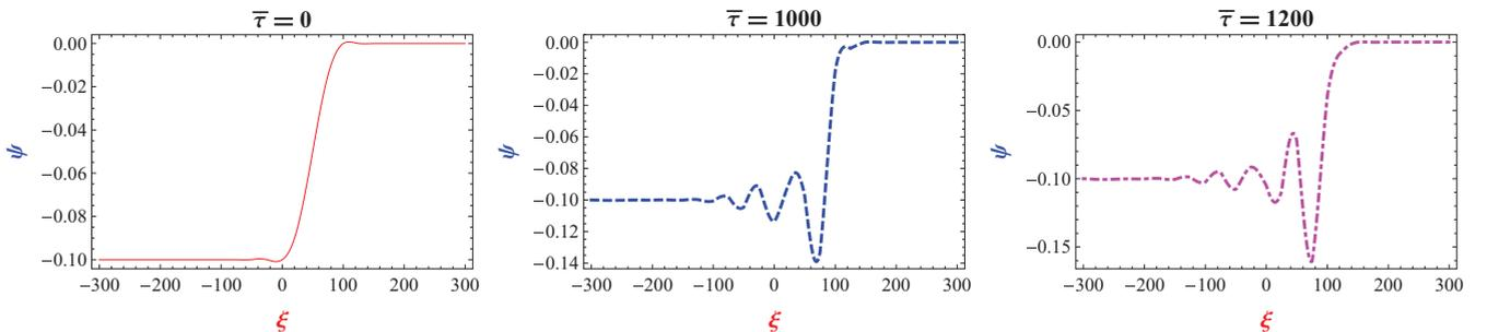
FIG. 1. (Color online) Evaluation of an oscillatory shock. The upstream value is  $U = 0.05$ . The plasma parameters are  $\alpha = 0.2$  and  $\nu = 0.1$ . At  $\bar{\tau} = 0, 1000, 1200$ . An oscillatory shock is fully developed at  $\bar{\tau} = 1200$ . Here we measure  $\xi$  in units of  $\lambda_{Dh}$  and time in units of  $\omega_{pc}^{-1}$ .
