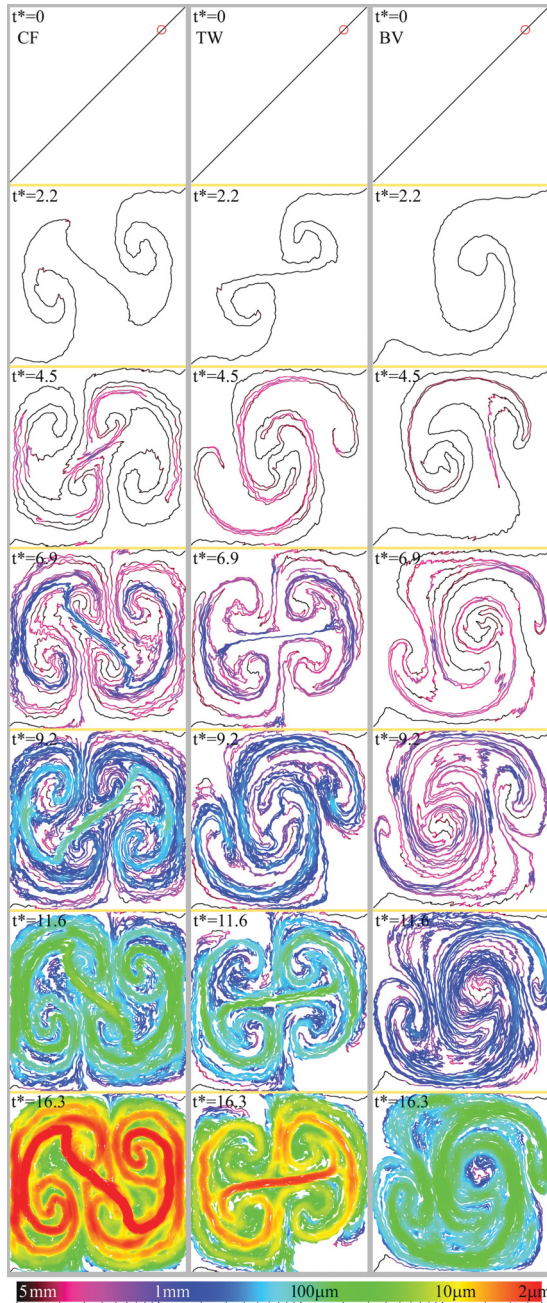
FIG. 9. (Color) The columns show the temporal advancement of a material line for the three sequences, from left to right: CF, TW, and BV. The color scale gives the striations' thicknesses d within measurement circles of diameter \phi = 1 cm, illustrated (in red) at t^* = 0 . The line tracked represents the interface between the numerical dyes in Fig. 7. Only the points for which the line's length from these points to the line's extremities is larger than \phi/2 are displayed.
