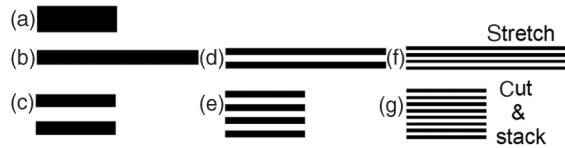
FIG. 11. Successive stretching, cutting, and stacking of material bands usually called the baker's map. The total length of the band is regularly multiplied by 2 and then grows exponentially as 2^n .
