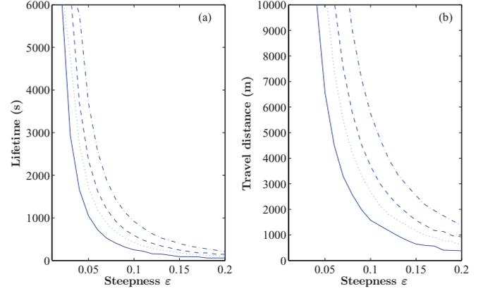
FIG. 10. (Color online) Lifetimes (a) and travel distances (b) of Peregrine-type wave structures vs steepness for  $\lambda = 100 \text{ m}$ , defined by amplification factors of 1.25 (dash-dotted), 1.50 (dashed), 1.75 (dotted), and 2.20 (solid).
