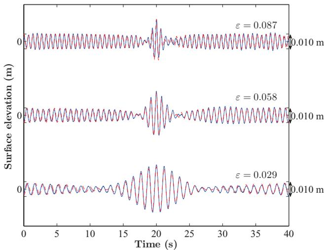
FIG. 6. (Color online) Comparison of measured surface heights at the position of maximum wave amplitude (solid line) with Peregrine soliton solution (dashed line) evaluated at  $X = 0$  for steepness 0.087, 0.058, and 0.029 by varying the wave number. The scaling parameter  $a_0 = 0.010 \text{ m}$ .
