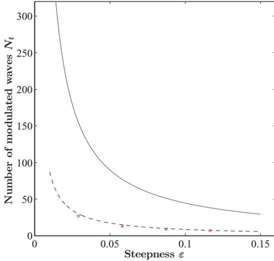
FIG. 7. (Color online) The number of modulated waves in time  $N_t$  vs steepness  $\epsilon$ . The value of  $N_t$  calculated for the Peregrine breather when the threshold amplitude is 0.99 (solid line) or 0.75 (dashed line). Crosses  $\times$  represent the experimental values obtained for a threshold amplitude of 0.75.
