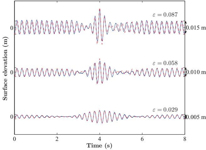
FIG. 5. (Color online) Comparison of measured (solid line) wave profiles at the position of maximum wave amplitude with theoretical Peregrine soliton solution (dashed line) evaluated at  $X = 0$  for steepness 0.087, 0.058, and 0.029 by varying the amplitude. The wave number  $k_0 = 11.6 \text{ m}^{-1}$ .
