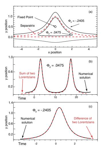
FIG. 1. (Color) (a) Potential contours of the Lorentzian bifurcation with parameter values b=c=1. (b) Numerical solution along the contour  $\Phi_0=0.0475$  compared to the sum of two Lorentzians. (c) Numerical solution along the contour  $\Phi_0=-0.2405$  compared to the difference of two Lorentzians.
