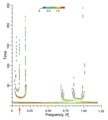
FIG. 2. (Color) Contours of y(t), with amplitude values indicated by the color bar, as a function of modulation frequency and time. Chaotic behavior is observed in two frequency intervals.
