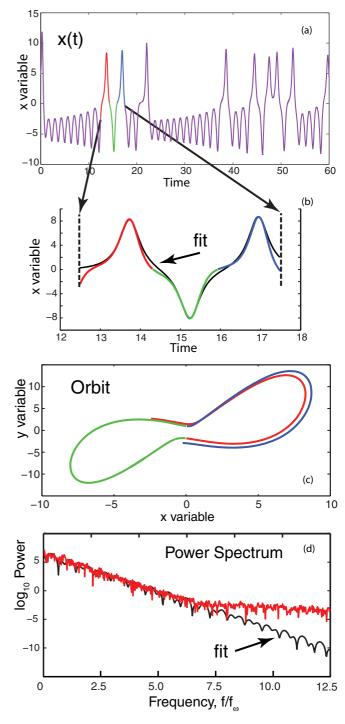
FIG. 4. (Color) (a) Time series for Lorenz model variable x shows intermittent pulses. (b) Color-coded time series is fit by a sum of three Lorentzian functions (black curve). (c) Phase-space trajectory of variables (y, x) is near the limit cycle of the attractor. (d) Frequency power spectrum of time series (red) compared to spectrum (black) of the sum of three Lorentzians.
