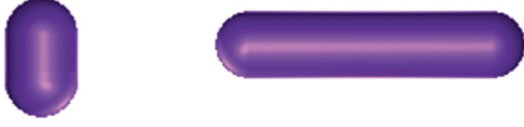
FIG. 10. (Color online) Spherocylinders composed of a cylinder with length L , capped at both ends with hemispheres with radius R . Left panel: a spherocylinder with aspect ratio L/R = 1 . Right panel: a spherocylinder with aspect ratio L/R = 5 .
