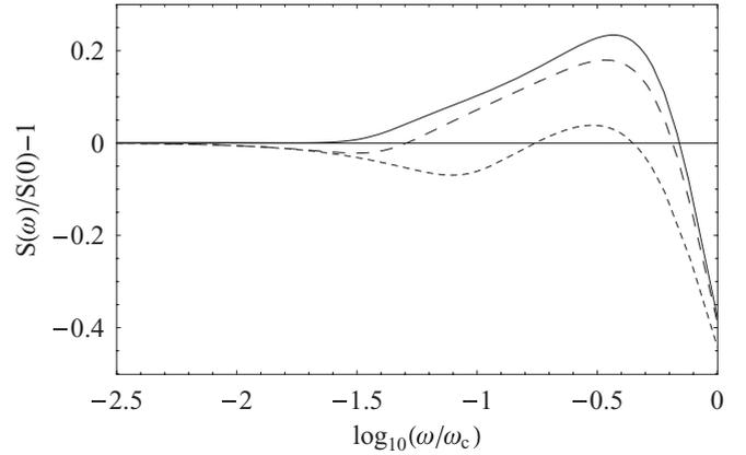
FIG. 2. Reduced spectral density  $S(\omega)/S(0) - 1$  as a function of  $\log_{10}(\omega/\omega_c)$  for a Brownian particle of radius  $a$  at distances  $h = 5a$  (solid curve),  $h = 7a$  (long dashes), and  $h = 9a$  (short dashes) from a planar wall with partial-slip boundary condition. The parameter values are listed in Sec. V.
