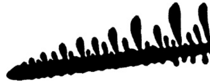
FIG. 4. Example of the crystal contour detection and the image binarization for the structure shown in Fig. 2 (160 s).
