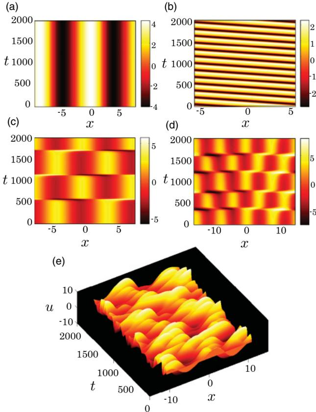
FIG. 2. (Color online) Spatio-temporal dynamics of the solution of Eq. (7). (a) Steady wave ( $L = 18.0$ ). (b) Traveling wave ( $L = 12.5$ ). (c) Heteroclinic oscillation ( $L = 13.7$ ). (d) Heteroclinic oscillation ( $L = 29.5$ ). (e) Turbulized dynamics ( $L = 21.5$ ). Here, we use the spectral algorithm with a fourth order exponential time differencing Runge-Kutta method (ETDRK4) [29], where the whole mode number is  $N = 512$ .
