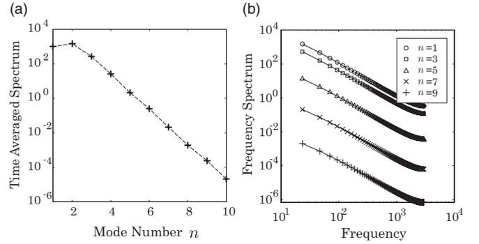
FIG. 3. (a) Time-averaged power spectrum. The spectrum higher than the  $n = 10$  mode continues to exponentially decrease (not shown here). (b) Frequency spectrum of low-wavenumber modes:  $n = 1, 3, 5, 7$ , and  $9$ . These are obtained by numerically solving Eq. (7) with the same parameter values as those used in Fig. 2(e).
