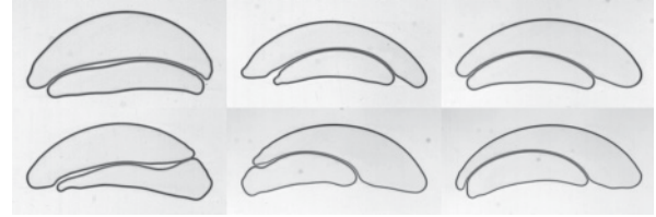
FIG. 5. Overview of different pairs of bubbles just prior to coalescence showing how the bubbles adapt their shapes to each other. Note that each pair of bubbles is shaped like a single big bubble ( Ar_1 \approx 11\,000 and Ar_2 \approx 7000 ).
