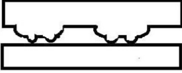
FIG. 1. This is a schematic illustration of the asperity hierarchy on the top surface sliding on a flat substrate (i.e., the bottom block). (Real asperities have arbitrary shapes, as opposed to the rectangular shapes shown in this schematic representation.) Each asperity of a given order has a number of (smaller) asperities of one order lower on its surface. In turn, each of these lower order asperities has a number of (smaller) asperities of one order lower. This continues until we reach the zeroth order asperity, whose surface consists of atoms. Only three orders of asperities are illustrated here.
