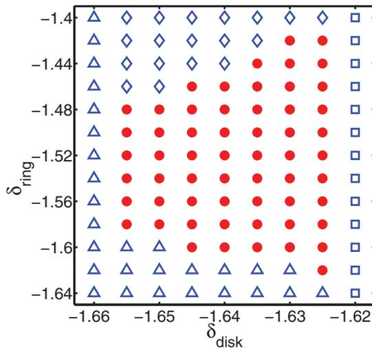
FIG. 2. (Color online) Phase diagram of patterns for  $\delta_{\text{disk}}$  vs  $\delta_{\text{ring}}$ . The circles denote the IRS patterns, the diamonds the unsteady patterns, the squares the intermediate patterns, and the triangles the no-excitation propagation patterns. Note that the IRS in Fig. 1(b) is the longest wave in our simulation, and longer waves with several wavelengths are not observed, even at a larger medium (with system size  $4096 \times 4096$  grid points).
