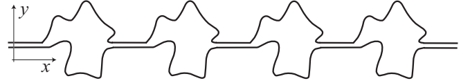
FIG. 2. A schematic plot of a periodic chain of chaotic billiards. The leads that connect the chaotic cavities have a width W such that if the wave number is k there are N = [Wk/\pi] modes that propagate along them. The cavity has an area A_c and the length of the unit cell is a , which we set to 1 unless we specify it otherwise. For the analysis of conductance the number of cells L is finite (here L = 4 ), the leftmost and rightmost leads extend to x minus and plus infinity, and we deal with a scattering system.
