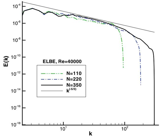
FIG. 3. (Color online) Energy spectrum at  $Re = 40000$ . ELBE simulations on grids  $110^3$  (double dot-dashed),  $220^3$  (dot-dashed) and  $350^3$  (solid line). Line with the slope  $-5/3$ : Kolmogorov's scaling.
