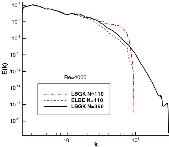
FIG. 2. (Color online) Energy spectrum at  $Re = 4000$ . Solid line: Resolved DNS [6] (LBGK, grid  $350^3$ ); Dashed: ELBE, grid  $110^3$ ; Dot-dashed: LBGK, grid  $110^3$ . Accumulation of energy at the short-wave end of the spectrum for LBGK is a precursor of numerical instability, which terminates the LBGK simulation on the grid  $100^3$ .
