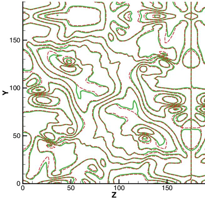
FIG. 1. (Color online) Isocontours of the  $z$  component of the velocity on a slice through the simulation domain at  $x = 20$ , at  $Re = 4000$ . Grid size  $350^3$ . One quarter of the slice is shown due to flow symmetry. Solid line: ELBE; Dashed: LBGK.
