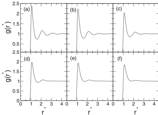
FIG. 2. The radial distribution function  $g(r^*)$  as a function of distance  $r^*$  at pressure  $P^* = 0.20 (> P_c^* \simeq 0.16)$  and six different temperatures (a)  $T^* = 1.02$ , (b)  $T^* = 1.12$ , (c)  $T^* = 1.26$ , (d)  $T^* = 1.36 (\approx T_w^*)$ , (e)  $T^* = 1.44$ , and (f)  $T^* = 1.58$ . As  $T^*$  increases along the isobaric path,  $g(r^*)$  shows that the peaks gradually decrease.
