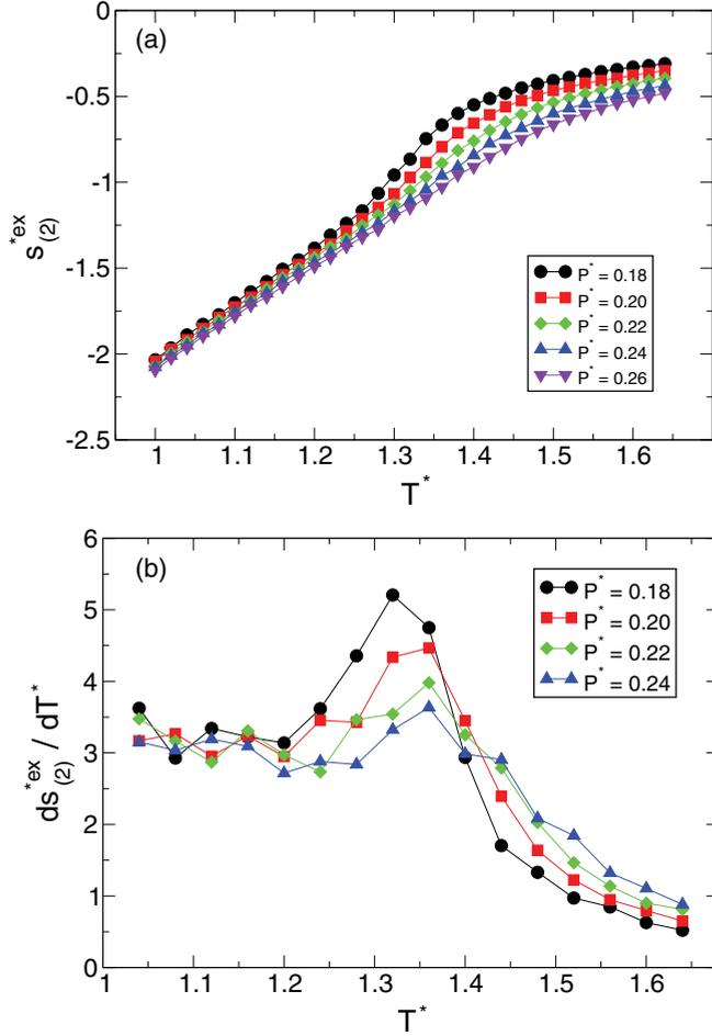
FIG. 4. (Color online) (a) The two-body excess entropy  $s_{(2)}^{*ex}$  and (b) the two-body excess entropy change  $ds_{(2)}^{*ex}/dT^*$  as a function of temperature  $T^*$  for different pressures in the supercritical region.  $ds_{(2)}^{*ex}/dT^*$  shows the maximum at the Widom temperature  $T_w^*(P^*)$ .
