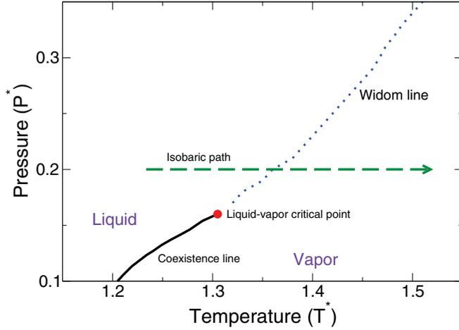
FIG. 1. (Color online) Phase diagram of the LJ fluid in the temperature-pressure ( $T^* - P^*$ ) plane. A black solid line is the liquid-vapor coexistence line. A red circle is the liquid-vapor critical point. Blue dots represent the locus of the isobaric specific heat maxima. A green dash line is the isobaric path ( $P^* = 0.20$ ) we used in this study. All data are taken from our simulation results.
