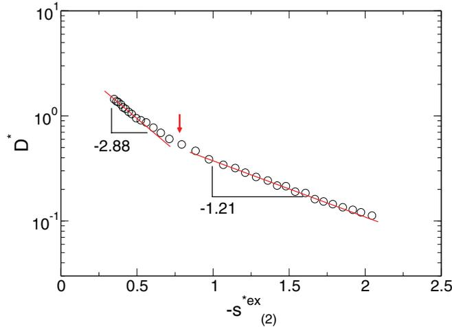
FIG. 6. (Color online) Shown in a semilog plot is the diffusion coefficient  $D^*$  versus the negative of the two-body excess entropy  $-s_{(2)}^{*ex}$  at  $P^* = 0.20 (>P_c^*)$ . It shows a crossover in the linear relationship between  $\ln D$  and  $s_{(2)}^{*ex}$ , given by  $D \propto \exp[Bs_{(2)}^{*ex}]$ . The parameter  $B$  is 2.88 at high temperature and 1.21 at low temperature. The arrow denotes the location of the Widom line.
