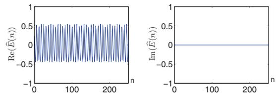
FIG. 5. (Color online) Real and imaginary parts of the function  $\widehat{E}(n)$  corresponding to one simulated trajectory of the stable harmonizable process. Since condition (12) is not satisfied, the process is not mixing. Length of the simulated trajectory  $N = 2^{12} + 1$ .
