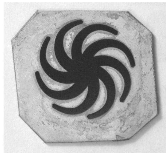
FIG. 5. Macroview of a special vortex pattern of a laser-processed area of an aluminum plate that causes stationary rotation of the liquid in the whole vessel. The diameter of the laser-treated area is 20 mm. The direction of rotation is counterclockwise.
