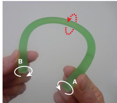
FIG. 4. (Color online) (Top) Geometric aspect of twist transport in a whirling rod:  $2\pi$  global rotation removes the  $4\pi$  axial twist. (Bottom) Simple demonstration with a rod bent into a half circle.
