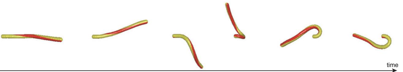
FIG. 2. (Color online) Trajectory of shape changes during the twirling-whirling transition. For  $\omega_0 > \omega_c$ , twirling (axial spinning) becomes unstable and the rod buckles to realize a large-amplitude whirling state. The snapshots here are obtained from our dynamic simulations for  $L/a = 30$  and  $\omega_0/\omega_c = 1.2$  [15,19].
