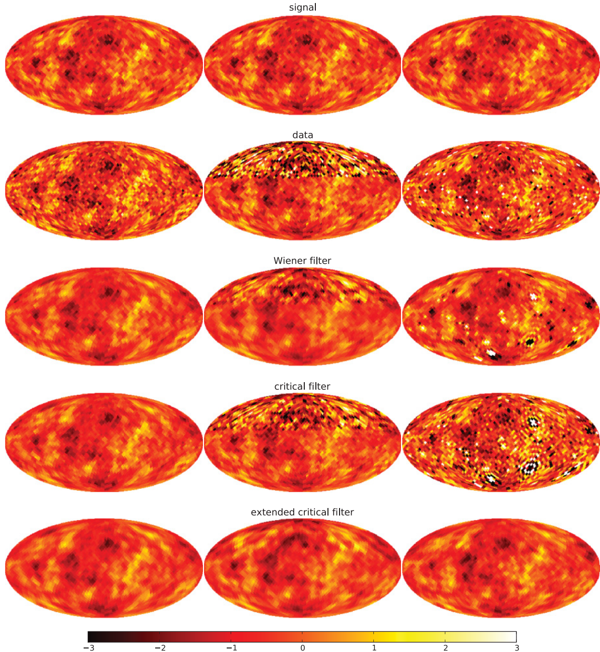
FIG. 2. (Color online) Comparison of different filter algorithms in the spherical case. Each column corresponds to a different setting. The signal, drawn from a power-law power spectrum, is the same in each case. The left column contains homogeneous noise, while in the middle column, the noise is suppressed in the southern third of the sphere and enhanced in the northern third, and in the right column the noise is enhanced in some individual pixels. The first row shows the signal realization and the second row the data. The third row shows the reconstruction using the Wiener filter formula, assuming the correct power spectrum and under the assumption of homogeneous noise; the fourth row shows the critical filter reconstruction, assuming the power spectrum to be unknown, but still assuming homogeneous noise. The last row shows the extended critical filter reconstruction in which both the signal power spectrum as well as the noise variance are assumed to be unknown.
