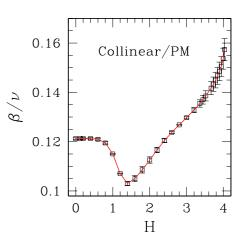
FIG. 4. (Color online) Finite-size magnetization exponent  $\beta/\nu$  along collinear-paramagnetic (PM) phase boundary. The range of fields  $0 \le H \le 4.027$  on the horizontal axis corresponds, respectively, to  $2.0820 \ge T \ge 0.75$  (see text). Each point is the result of fitting finite-size data in the range  $12 \le N \le 20$  to a single-power law  $\langle M^2 \rangle^{1/2} \sim N^{1-\beta/\nu}$ . See Eqs. (8) and (14).
